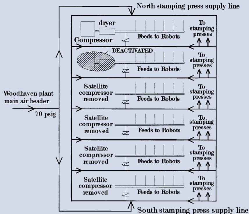
Review of the design characteristics of the robot's vacuum cup flow venturi determined that they would operate satisfactorily with the pressure available from the main header (about 70 psig). Five of the robots already had a supply line from the main header in parallel with the discharge piping from the high pressure satellite compressor. These five were reconfigured to receive air from the main header.
