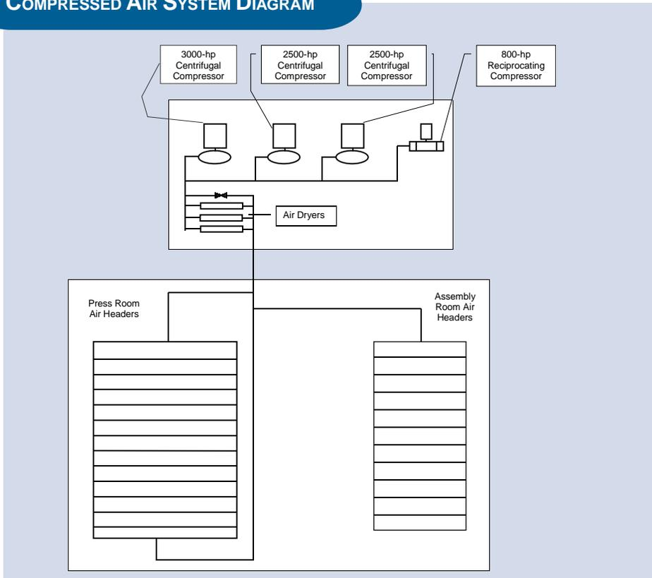
lower. It was possible to lower the compressor discharge pressure settings significantly, and the average main header pressure went from 75 psig to 70 psig. This change not only reduced the amount of energy that was required to produce the compressed air (see text box), but also reduced artificial demand (see text box), which contributed to lower compressed air and energy consumption.
